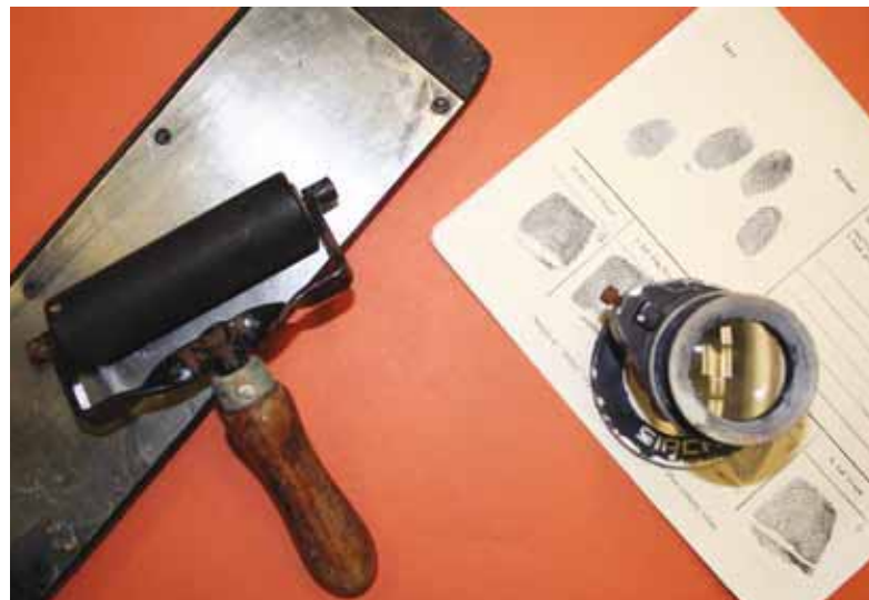
Equipment used in the early 1900s comprised a roller, metal slab, hand-held magnifying glass and fingerprint form.
