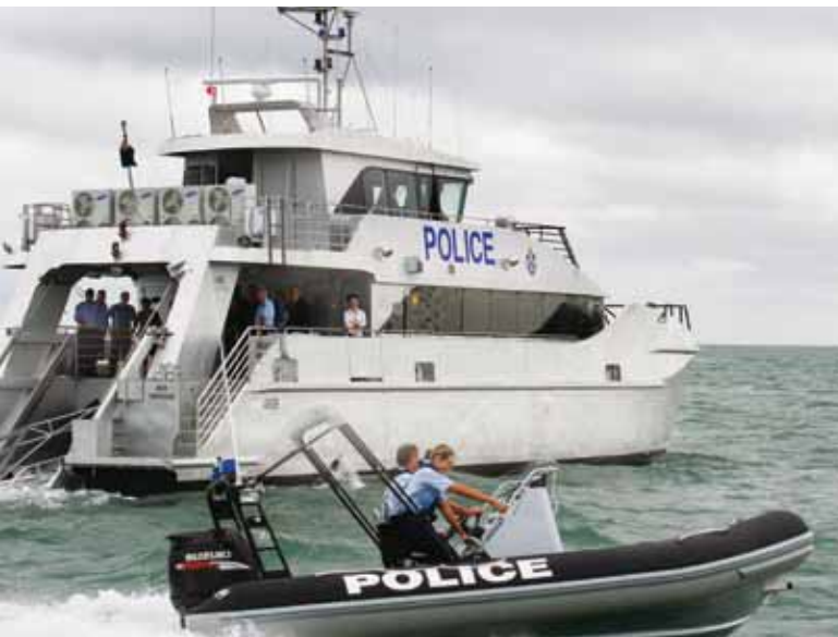
Below—The Lyle M Hoey makes its debut in Queensland waters in April 2009, launching a new era of water policing. It is one of three purpose-built catamarans designed to act as an independent forward command post. The Rigid Hull Inflatable Boat (foreground) can be rapidly deployed from the cradle between the twin hulls of the main vessel.
